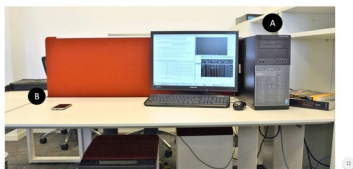
Figure 1. A typical exfiltration scenario. A compromised computer (A) - without speakers, and with audio hardware disabled - transmits sensitive information via acoustic signals. This information is received and decoded by a nearby mobile phone (B)
